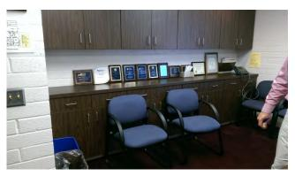
requires a 5-foot diameter turn around space. The existing cabinets are 36-inches tall; the height of the cabinets must not exceed 34 inches. The room is deficient in these areas.
