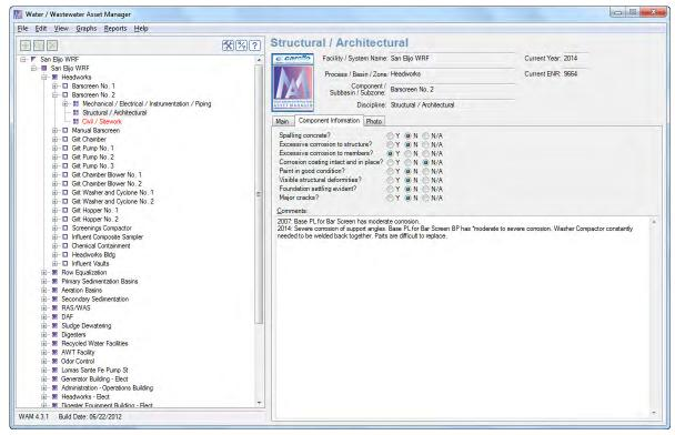
Figure 4.3 Component Section of Structural / Architectural Discipline Data for Barscreen No. 2
