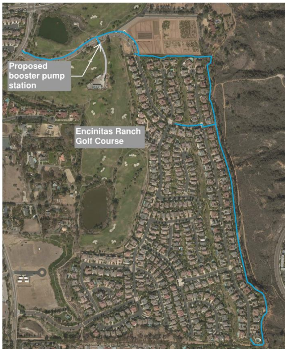
Figure 1 - Proposed pipeline alignment
